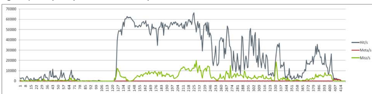
Figure 6) Example of per-second rate of requests served from Flash Cache and disks.
