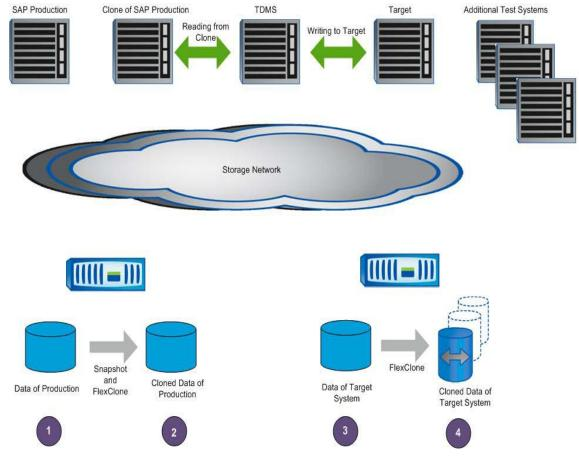
Figure 2) NetApp storage in an SAP TDMS environment.
