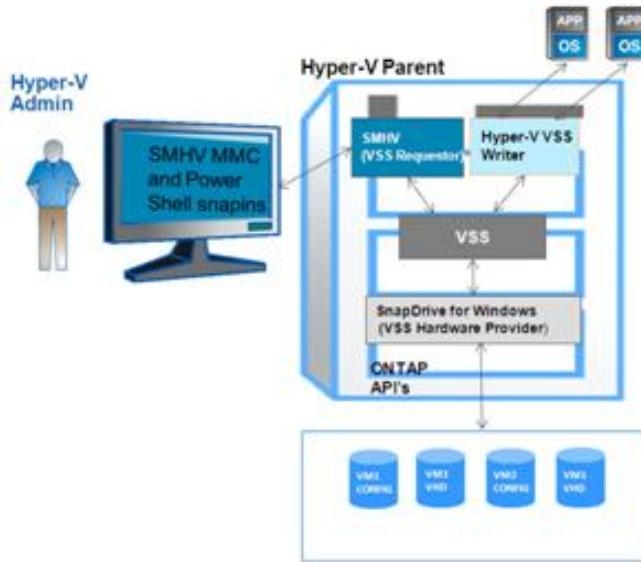
Figure 26 represents a high-level overview of the typical SMHV architecture on the primary site storage and will be used in detailing the backup process flow for application-consistent backups.
