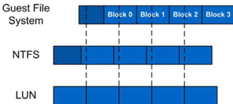
Figure 17) Guest OS and NTFS file system are aligned with the NetApp storage array blocks.
