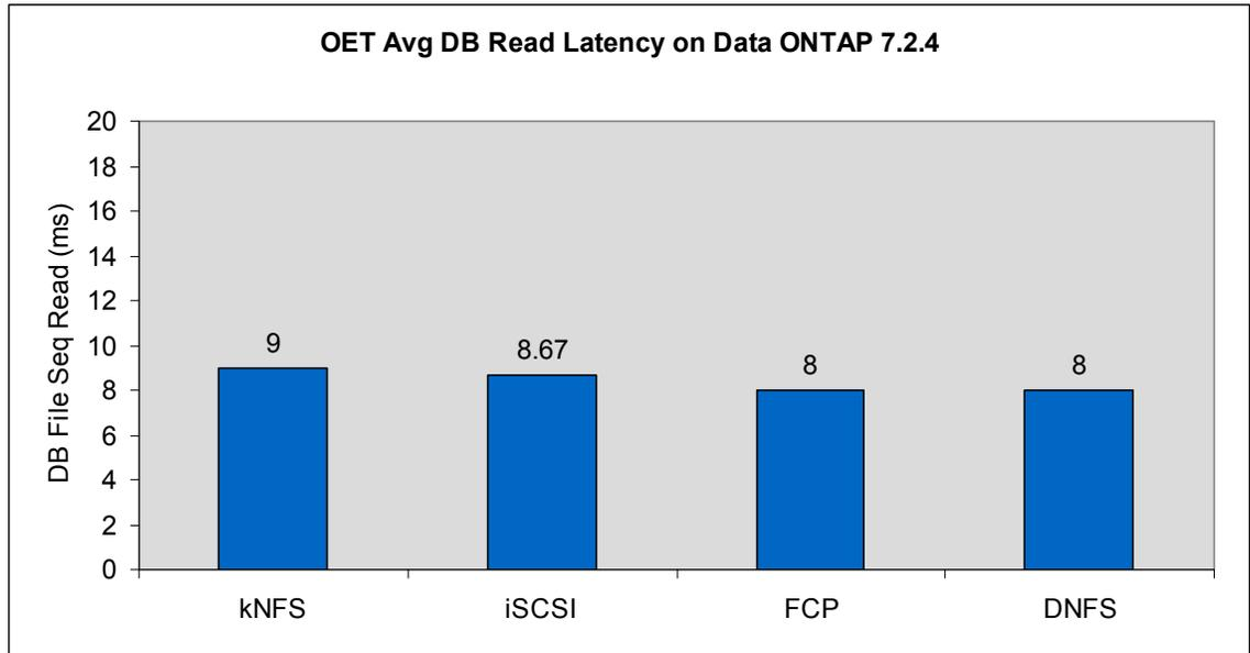
Figure 10) Average Oracle DB single-block read latency by protocol on Data ONTAP 7.2.4 (lower numbers are better).
