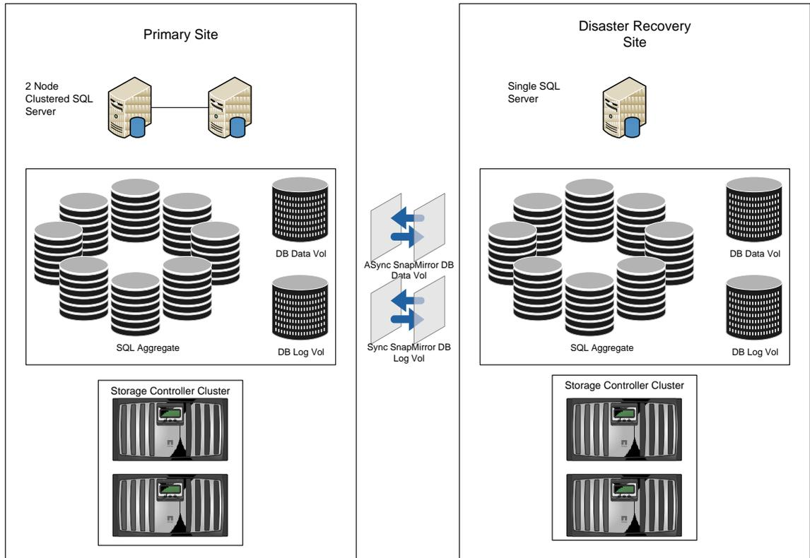
The following diagram shows the basic architecture used in this scenario using SnapMirror to asynchronously replicate data volumes and synchronously replicate log volumes
