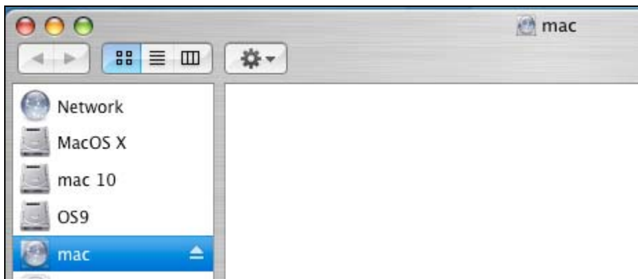
Figure 15) The .snapshot folder is not shown in the Finder on NFS-mounted volumes...
