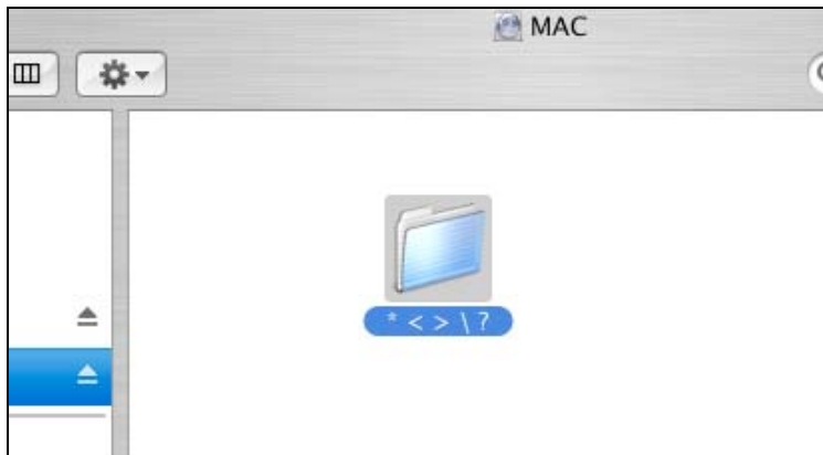
Figure 1) A folder name with “invalid” characters in an SFM AFP volume on a Mac client...
