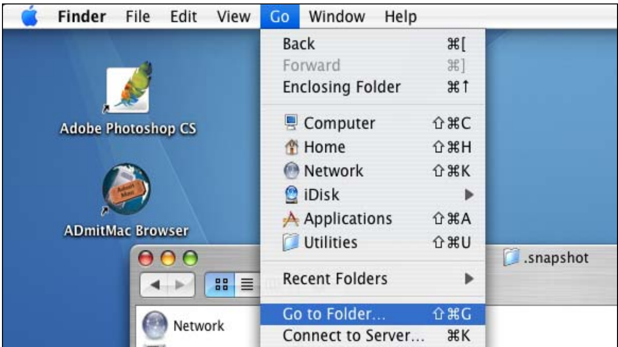
Figure 17) To restore from a Snapshot copy using Finder on NFS mounts, use “Go to Folder”...
