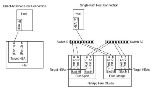
Figure 6-01. Direct connect and single-path host connection.
