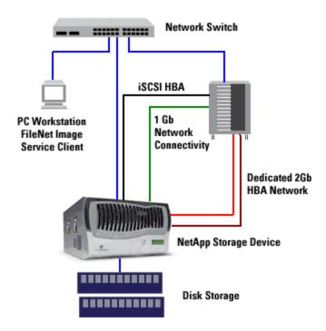
Figure 4-31. Simple Storage Area Network Configuration.
