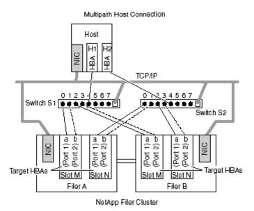
Figure 6-02. Multipath host connection with NetApp storage system cluster.
