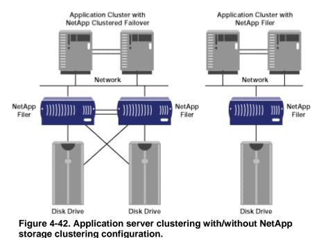
In a FileNet customer environment, the operating system can host both Image Services and the database server, or the database can be run on a separate, remote server connected to the storage. The design diagram is below shows how the FileNet solution integrates with storage. In Network Appliance Inc.
