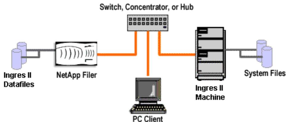
As shown in the network diagram, we recommend that you dedicate at least one private network connection between the Ingres II UNIX server machine and the filer. This can be done using a cross-over cable on most networking topologies (fast Ethernet and gigabit Ethernet being two examples we have tested successfully).
