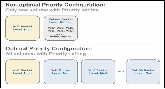
Figure 6) Priority Configuration with Processing Buckets
